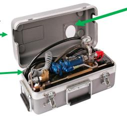
View window for pressure reading during swaging
